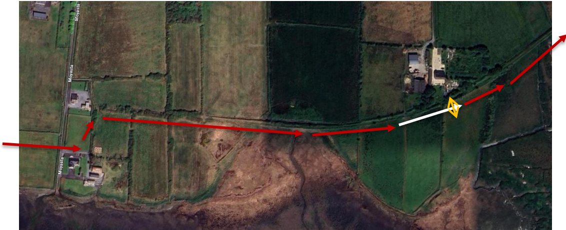
Figure 4-12 Proposed greenway route marked in red arrows and footbridge marked in orange arrow. Section that may require earth retaining measures marked in white arrow.
