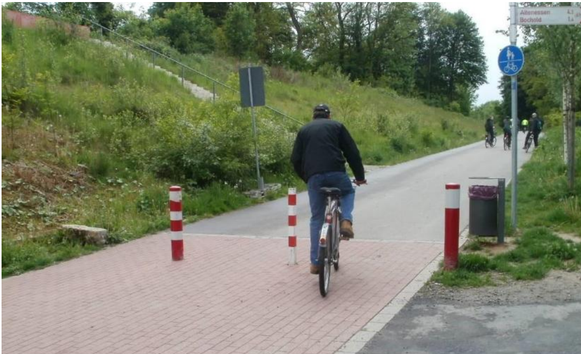
Figure 4-35 Simple Bollard Access - Generous width (Essen, Germany)
